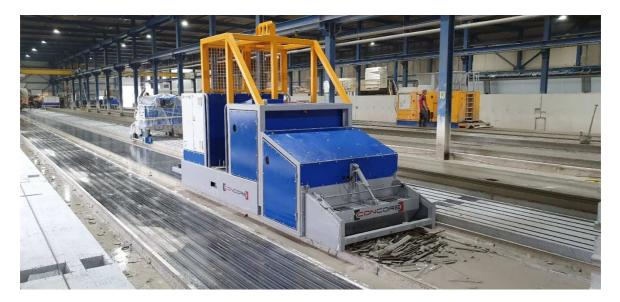
Preparing beds before casting is an labour intensive work, The Concore multifunction machine is therefore one of the most cost saving machines. It's not only saving on labour but also in there will be a big difference in the time preparing the beds. Therefore the return of investment on a Concore multifunction machine will be a very short time.
