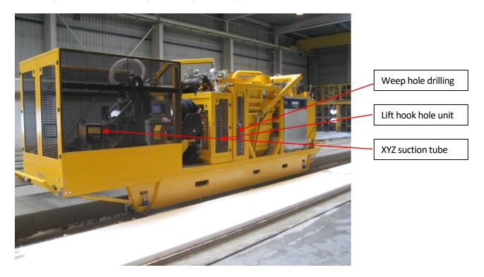
Semi-automatic operated Aspirator machine with Hook prepare unit and weep hole unit.
