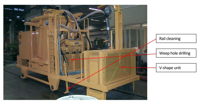
Manual operated Aspirator machine with removable hopper for emptying. The machine as shown is provided with rail cleaning, weep hole drilling and a solid V shape maker. The V-shape maker unit can also produce any other shape.
