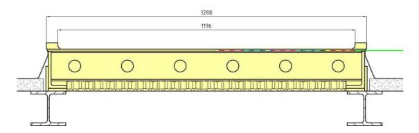
The Concore casting beds are delivered complete with heating pipes and insulation.
